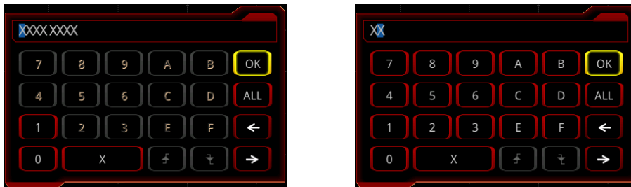
(a) Virtual Keypad for Binary Data Bit (b) Virtual Keypad for Hex Data Bit Figure 5-15 Virtual Keypad for Data Bit Settings
